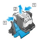
7 Attach a new staple case to the **Saddle Staple Cartridge**.
