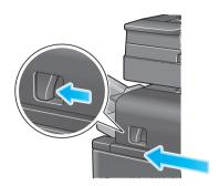
2 Pull the Punch Kit Release Lever [FS2] in the arrow direction, and open the Punch Kit.
