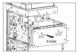
6 Unfasten 4 bolts to remove the interior frame from the device.
