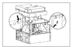
Install the Wifi module into the device and use the clamp to secure it as in the figure.
