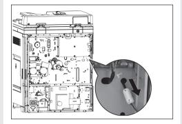
11 Connect the cable of Wifi module with the clamp from step 6 and assemble it into the device.
