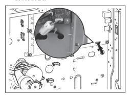
Fasten 6 bolts to secure the left cover back to the device.
