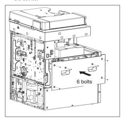
Fasten 14 bolts to assemble the rear cover back to the device.
