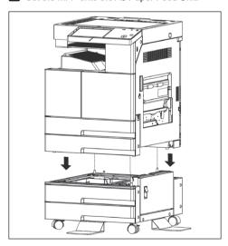
Remove the upper Tray [F] from the MFP. (When removing the tray, adjust the side fence to the A5 paper position first.)
