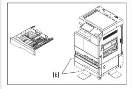
Place the upper Tray back to the MFP. (When setting the tray, adjust the side fence to the A5 paper position first.) 10 Remove the rear cover [G](14 bolts) from the MFP.
